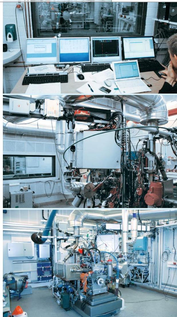
AVL Raptor including a dSPACE system can control, for example, a single-cylinder test bench for gasoline engines with a fully flexible valve system.
