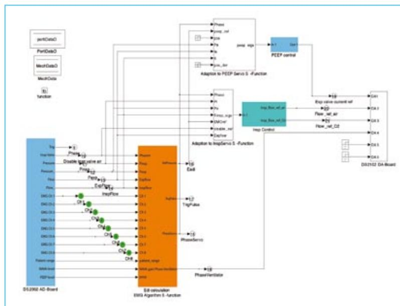
Figure 4: Simulink® model for EMG control of SERVO-i.
